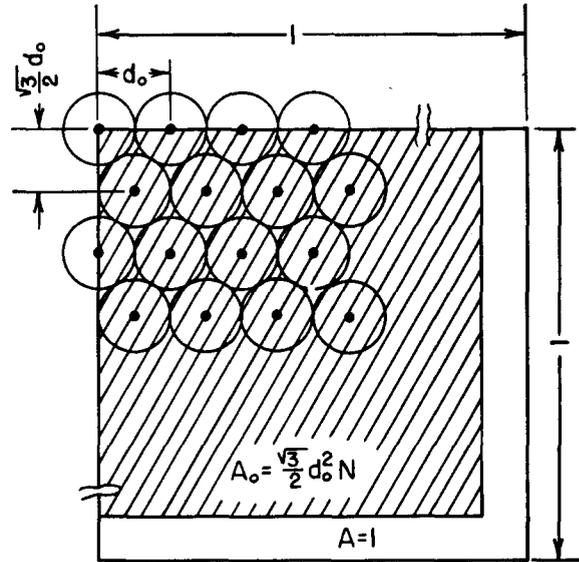
FIG. 3. The close-packed arrangement for determining  $A_0$ .
