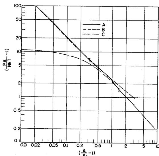
FIG. 4. A plot of  $(PA/NkT) - 1$  versus  $(A/A_0) - 1$ . Curve A (solid line) gives the results of this paper. Curves B and C (dashed and dot-dashed lines) give the results of the free volume theory and of the first four virial coefficients, respectively.
