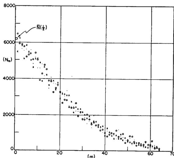
FIG. 5. The radial distribution function  $N_m$  for  $\nu = 5$ ,  $(A/A_0) = 1.31966$ ,  $K = 1.5$ . The average of the extrapolated values of  $N_{\frac{1}{2}}$  in  $\bar{N}_{\frac{1}{2}} = 6301$ . The resultant value of  $(PA/NkT) - 1$  is  $64\bar{N}_{\frac{1}{2}}/N^2(K^2 - 1)$  or 6.43. Values after 16 cycles,  $\bullet$ ; after 32,  $\times$ ; and after 48,  $\circ$ .
